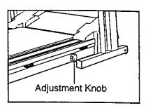
platform, turn the adjustment knob clockwise. To decrease the firmness, turn the knob counterclockwise. Note: The faster you run on the treadmill, the firmer the walking platform should be. If the walking platform is not adjusted correctly, the treadmill may bounce excessively.
